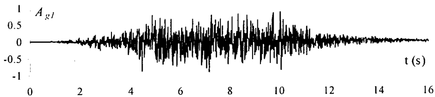
Fig. 4.1 Simulated ground acceleration A_{g1} according to KT model
