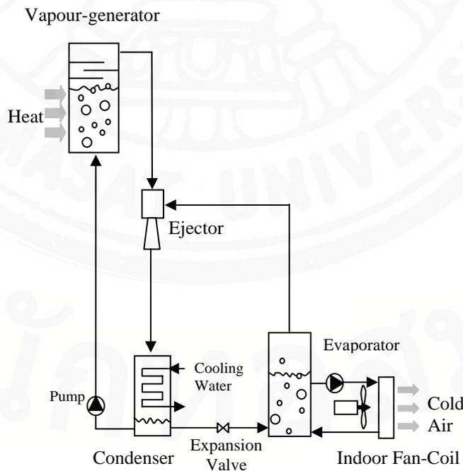
b) A typical ejector refrigeration cycle
