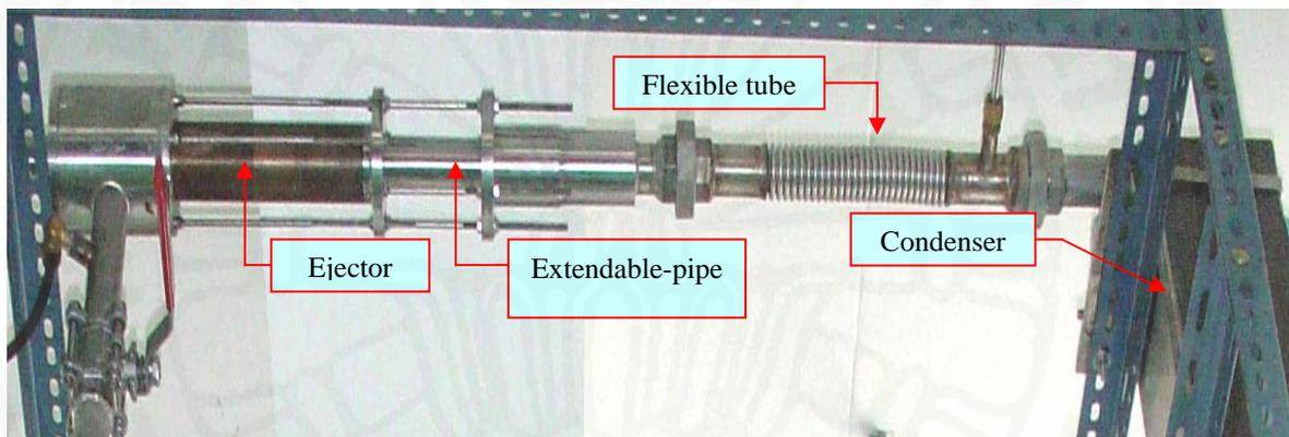
**Figure 3.3** Connection of the ejector in the experimental refrigerator.
