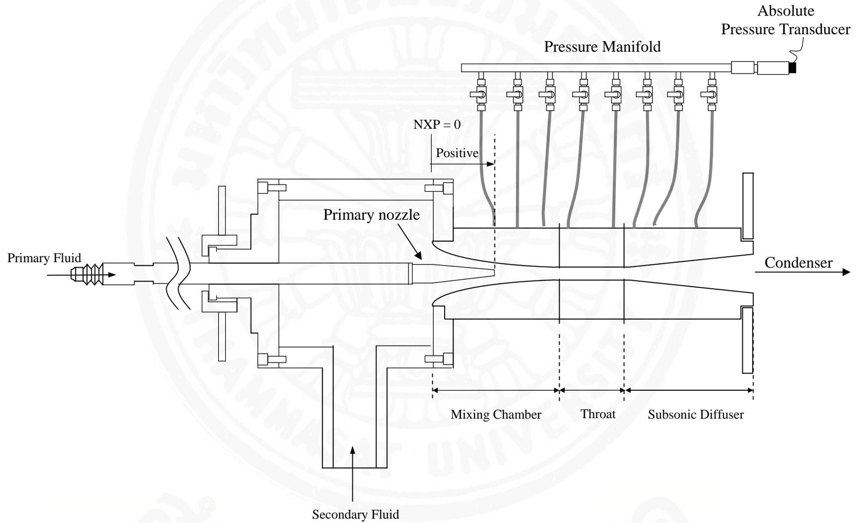
**Figure 3.5** Schematic Diagram of Experimental R141b Ejector.
