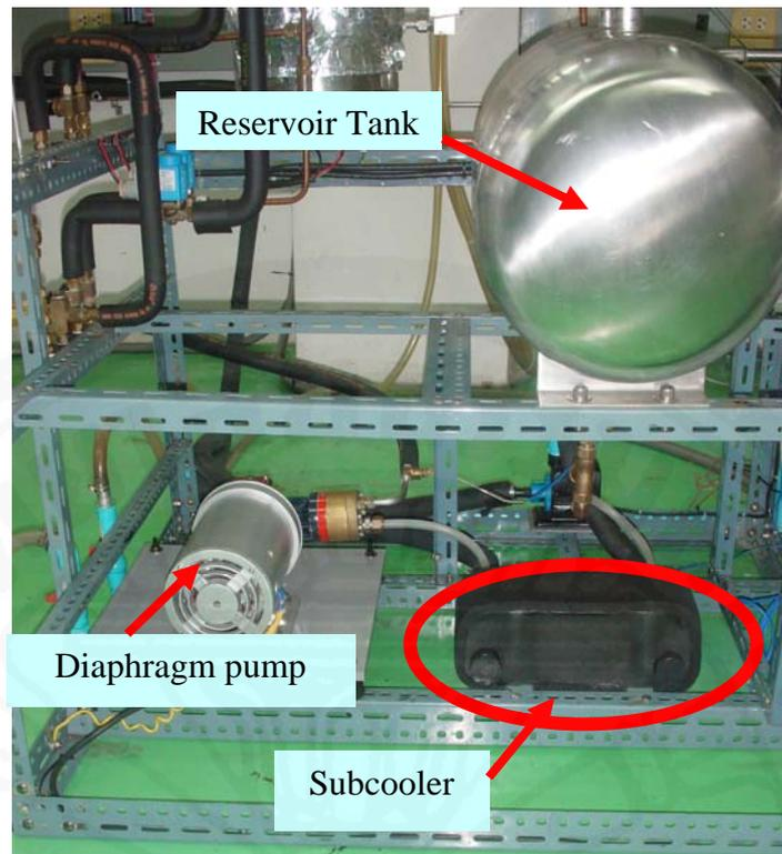
**Figure 3.4** The pumping system with the subcooler.
