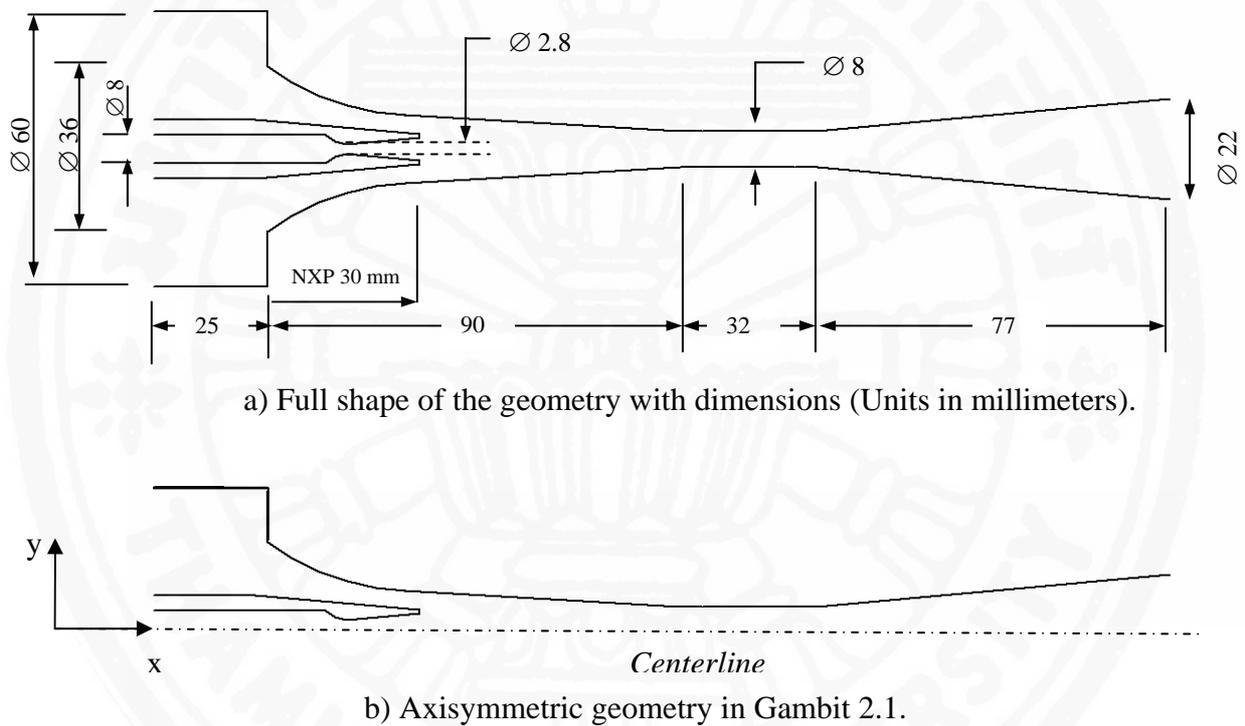
a) Full shape of the geometry with dimensions (Units in millimeters).
