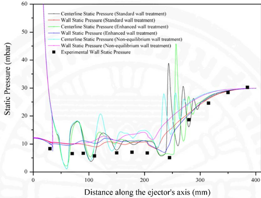
a) At  $T_p = 130\text{ }^\circ\text{C}$ ,  $T_s = 10\text{ }^\circ\text{C}$  and  $P_b = 30\text{ mbar}$ .
