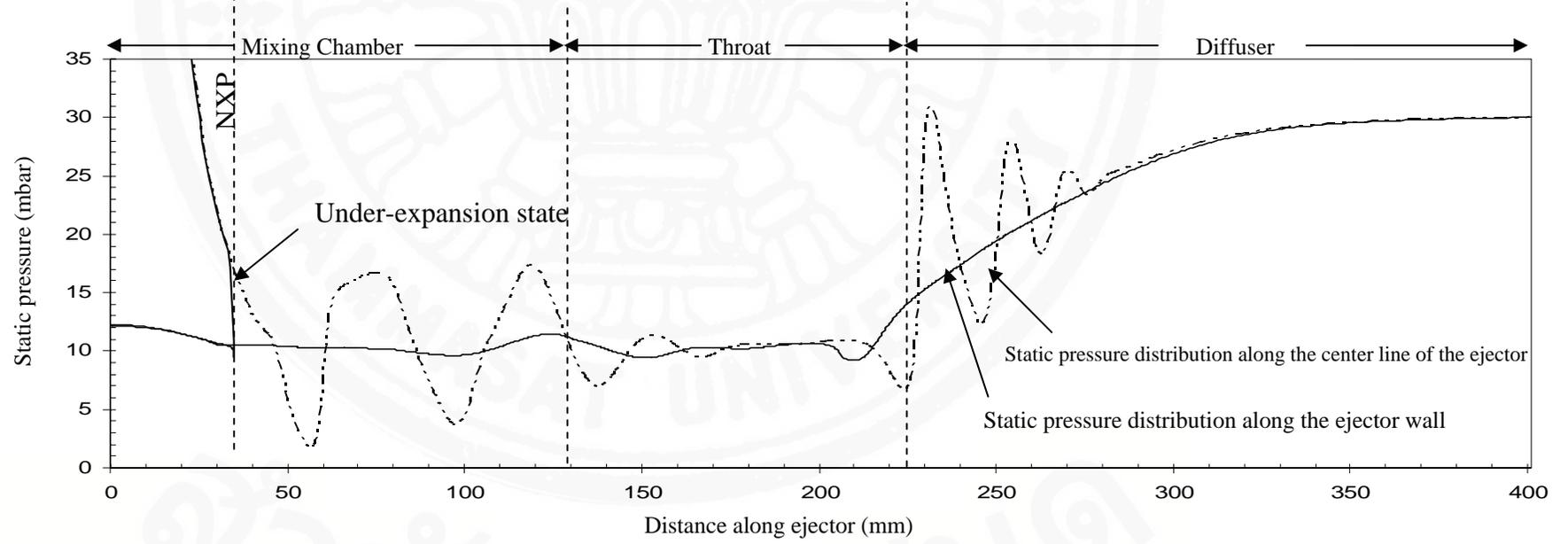
b) Static pressure distribution of the steam ejector
