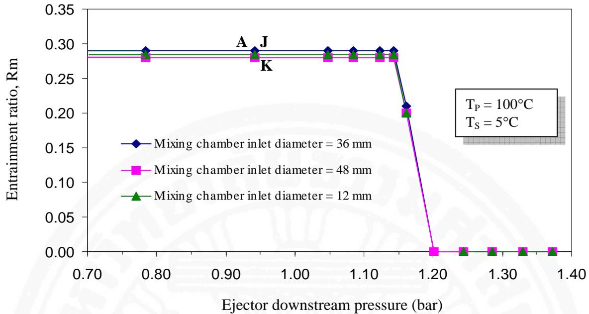
**Figure 8.3** Performance characteristics of the R141b ejector, effect of mixing chamber inlet diameter.
