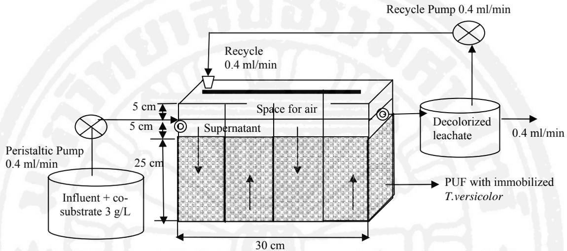
**Figure 3.1** Vertical flow baffled bioreactor
