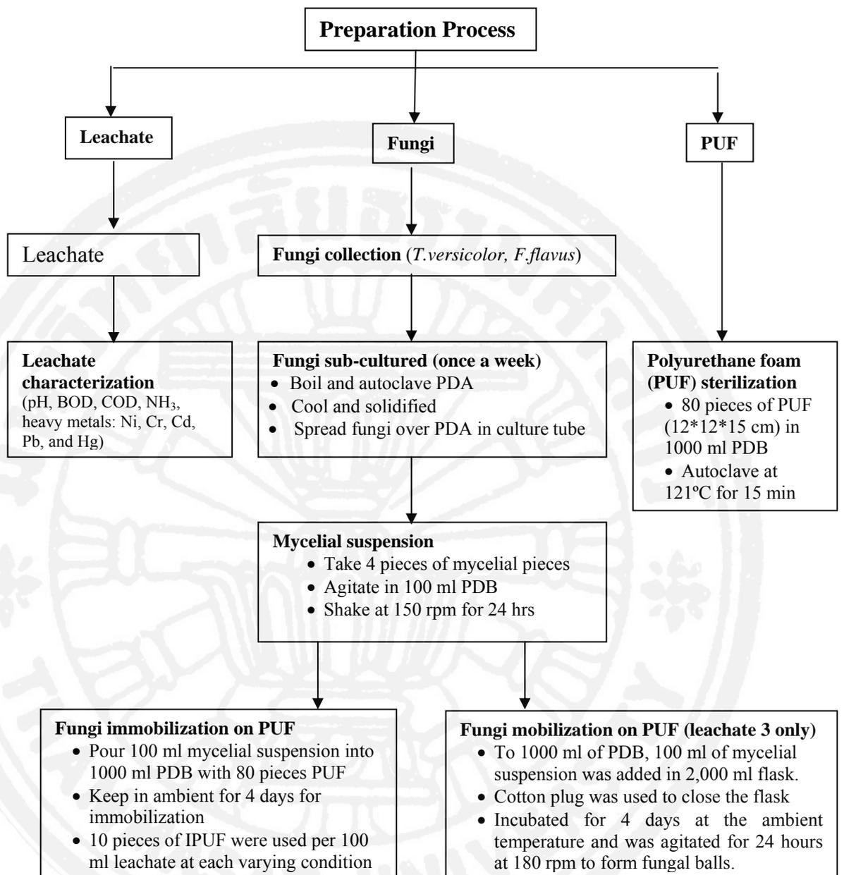
**Figure 3.2** The overview of the preparation process
