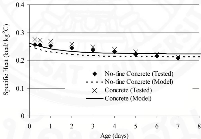
Fig 5.7 Comparison between predicted and Brown and Javid's test results specific heat of no-fine concrete and concrete
