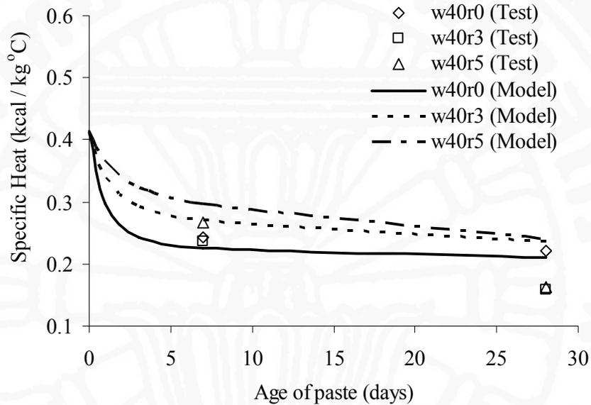
Fig 5.4 Comparison between predicted and test results of specific heat of cement-fly ash pastes with fly ash replacement ratios of 0, 0.3 and 0.5, and  $w/b = 0.40$
