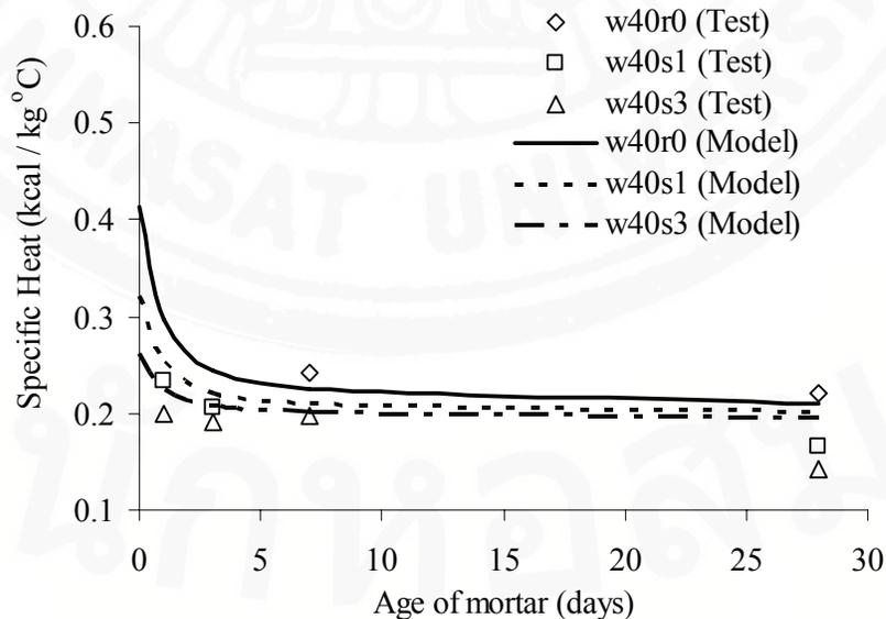
Fig 5.5 Comparison between predicted and test results of river sand mortars with  $s/b = 0, 1$  and  $3$ , and  $w/b = 0.40$ .
