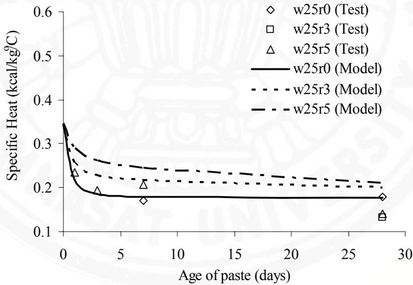
Fig 5.3 Comparison between predicted and test results of specific heat of cement-fly ash pastes with fly ash replacement ratios of 0, 0.3 and 0.5, and  $w/b = 0.25$
