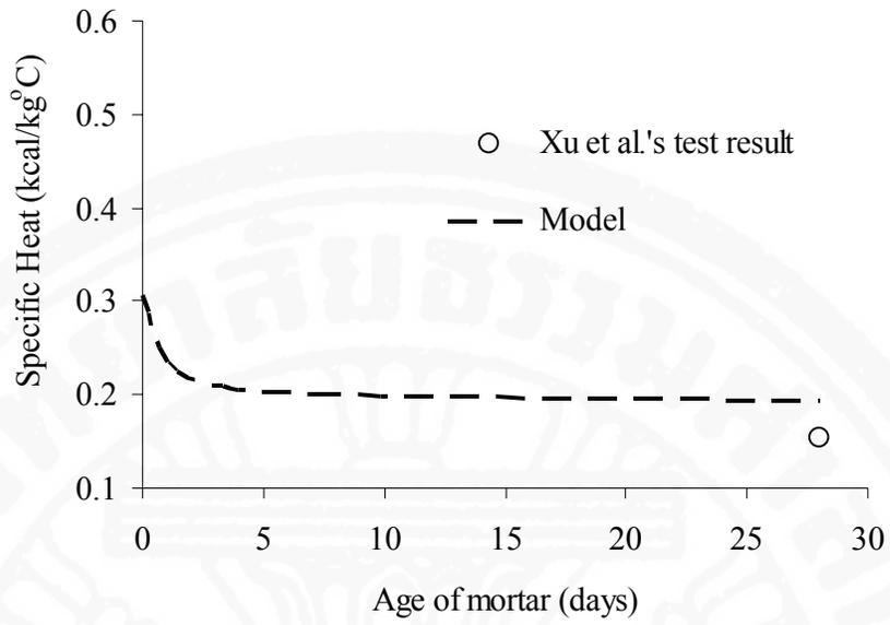
Fig 5.8 Comparison between predicted and Xu et al.'s test result of river sand mortar with  $s/b = 1$ , and  $w/b = 0.35$ .
