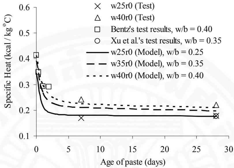
Fig 5.2 Comparison between predicted and authors' and other researchers' test results of specific heat of cement pastes with  $w/b = 0.25, 0.35$  and  $0.40$
