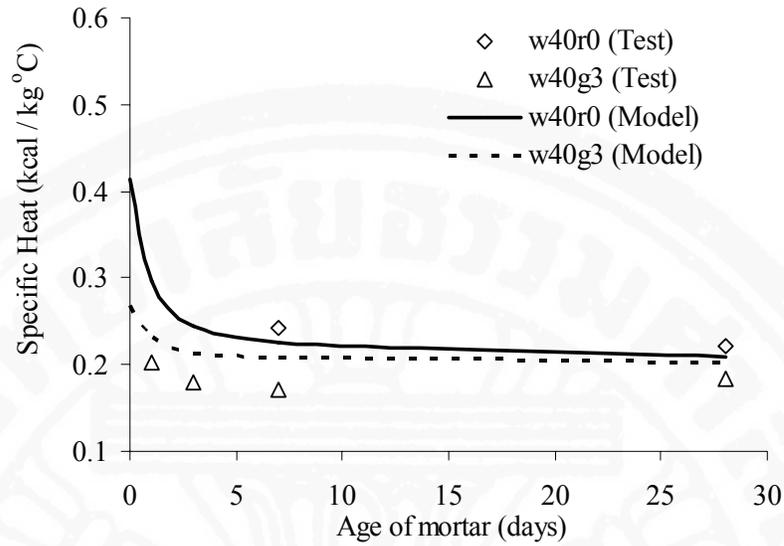
Fig 5.6 Comparison between predicted and test results of crushed limestone sand mortars with sand to binder ratios of 0 and 3, and  $w/b = 0.40$
