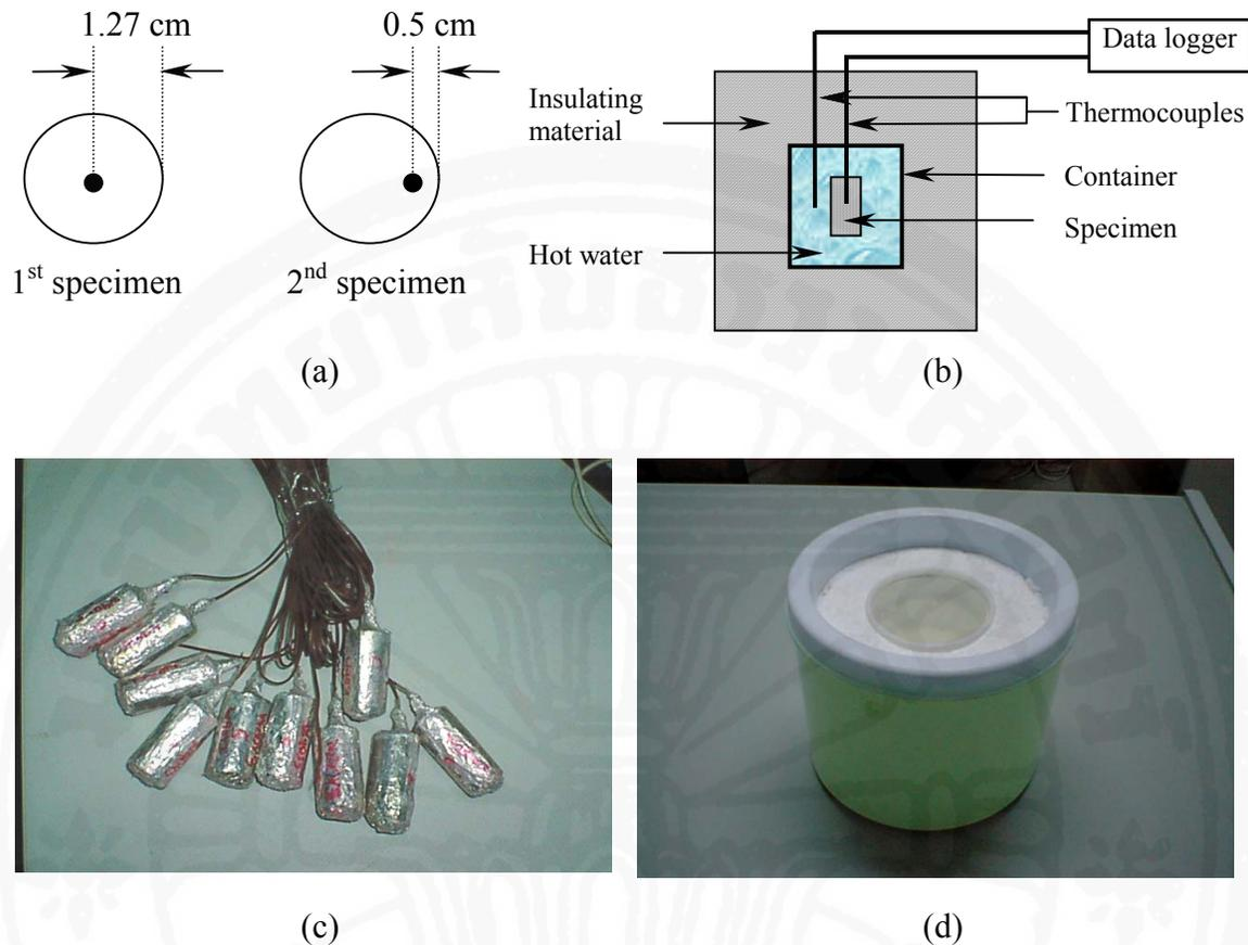
Fig 5.1 Apparatus for testing the specific heat (a) Positions of thermocouples, (b) Schematic illustration, (c) Sealed Specimens, (d) Insulated Container
