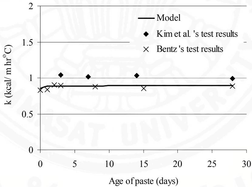
Fig. 6.9 Comparison between Kim et al.'s test results, Bentz's test results and  $k$  model of cement paste,  $w/b = 0.4$
