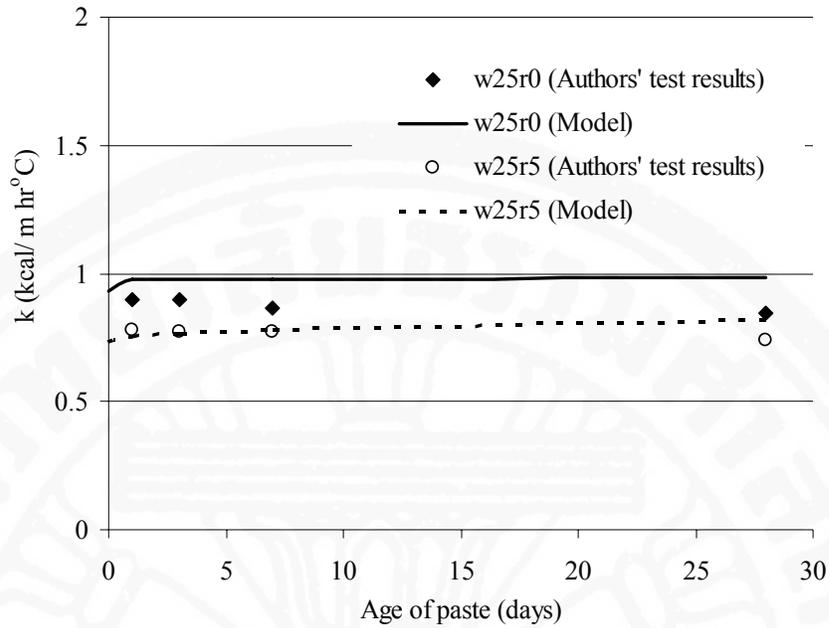
Fig. 6.5 Test and predicted results of  $k$  of pastes with  $w/b = 0.25$  and fly ash replacement ratio of 0 and 0.5
