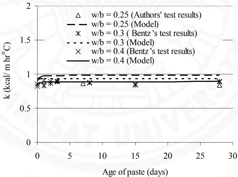
Fig. 6.6 Test and predicted results of  $k$  of pastes with  $w/b = 0.25, 0.3$  and  $0.4$
