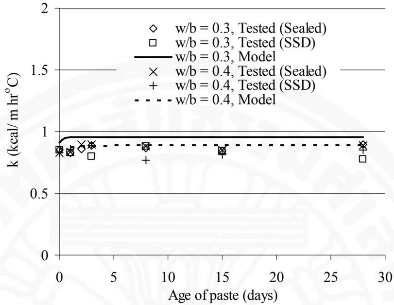
Fig. 6.10 Comparison between Bentz's test results and  $k$  model of cement paste,  $w/b = 0.3$  and 0.4
