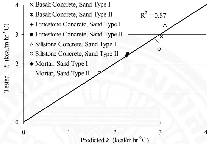
Fig. 6.12 Comparison between Khan’s test results and  $k$  model of mortars and concrete
