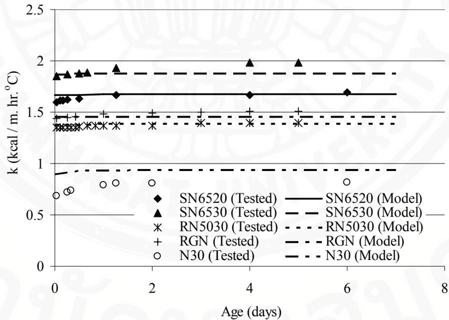
Fig. 6.11 Comparison between Toyokazu et al.'s test results and  $k$  model of paste, mortars and concrete
