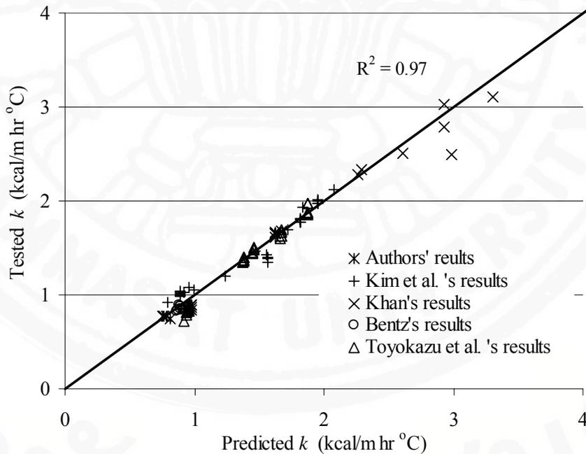
Fig. 6.14 Comparison between the predicted and the tested values of  $k$  measured by the authors' and all other referred data
