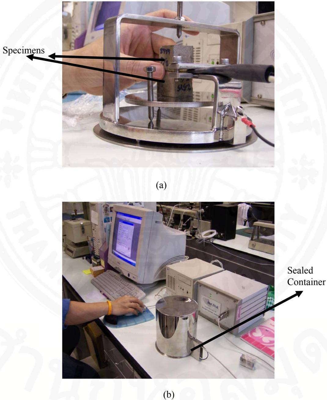
Fig. 6.1 Apparatus for Testing Thermal Conductivity (a) setting of specimens, (b) testing of specimens
