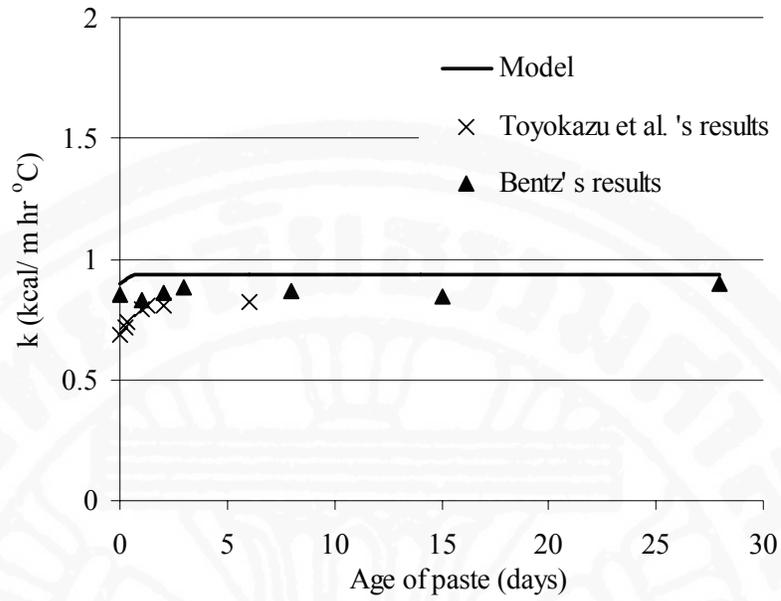
Fig. 6.8 Comparison between Toyokazu and Yoshiro's test results, Bentz's test results and  $k$  model of cement paste,  $w/b = 0.3$
