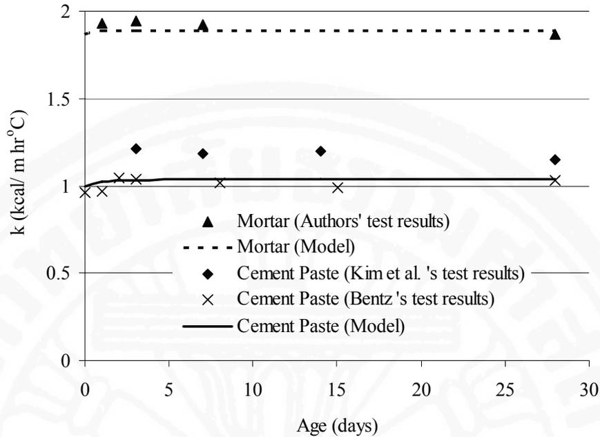
Fig 6.7. Test and predicted results of  $k$  of pastes with  $w/b = 0.4$  and mortar with  $w/b = 0.4$ ,  $g/b = 2$
