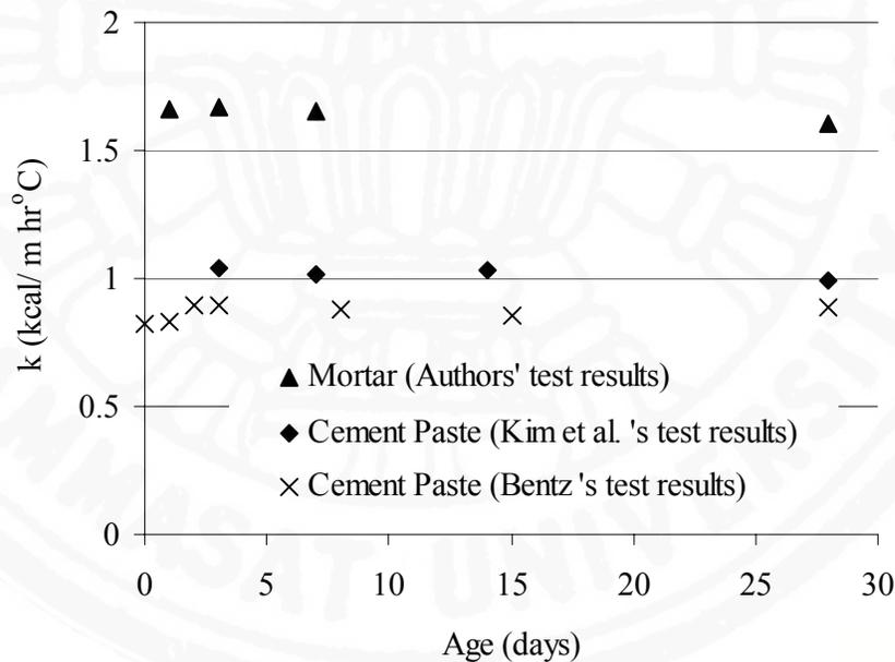
Fig 6.4. Test results of  $k$  of pastes with  $w/b = 0.4$  and mortar with  $w/b = 0.4$ ,  $g/b = 2$
