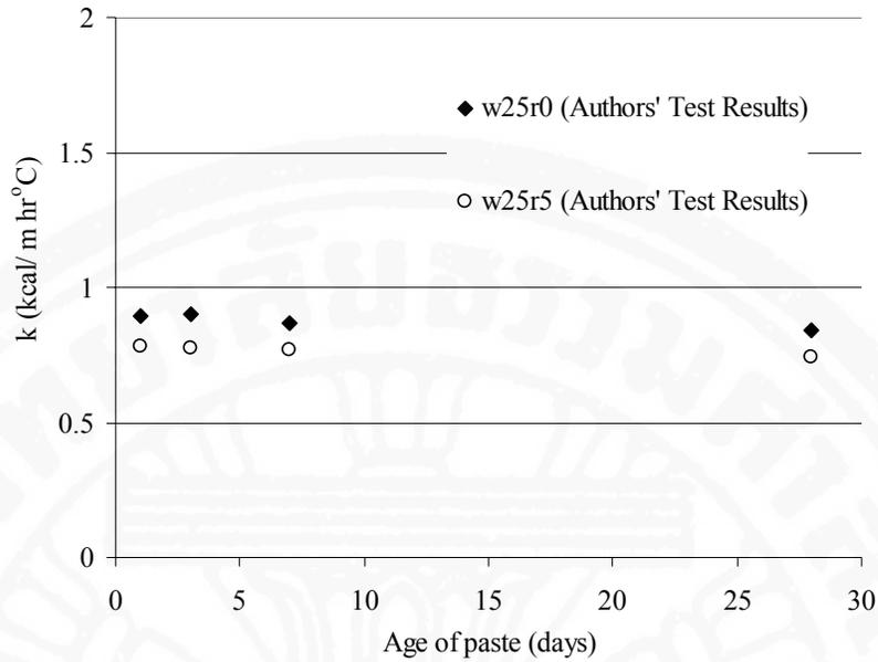
Fig. 6.3 Test results of  $k$  of pastes with  $w/b = 0.25$  and fly ash replacement ratio of 0 and 0.5
