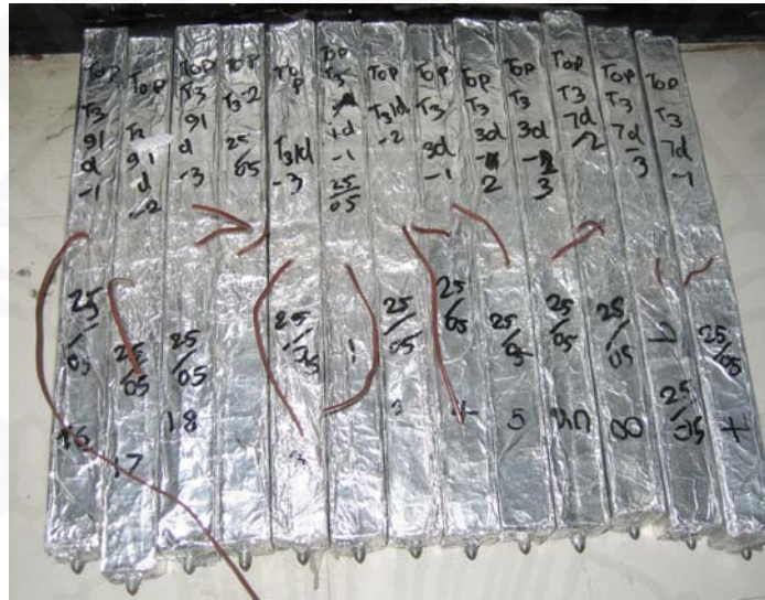
Fig. 7.1 Example of the wrapped cement – fly ash paste and mortar specimens
