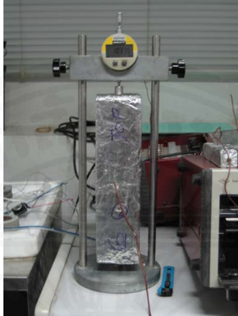
Fig. 7.3 Measurement of length change of a concrete specimen
