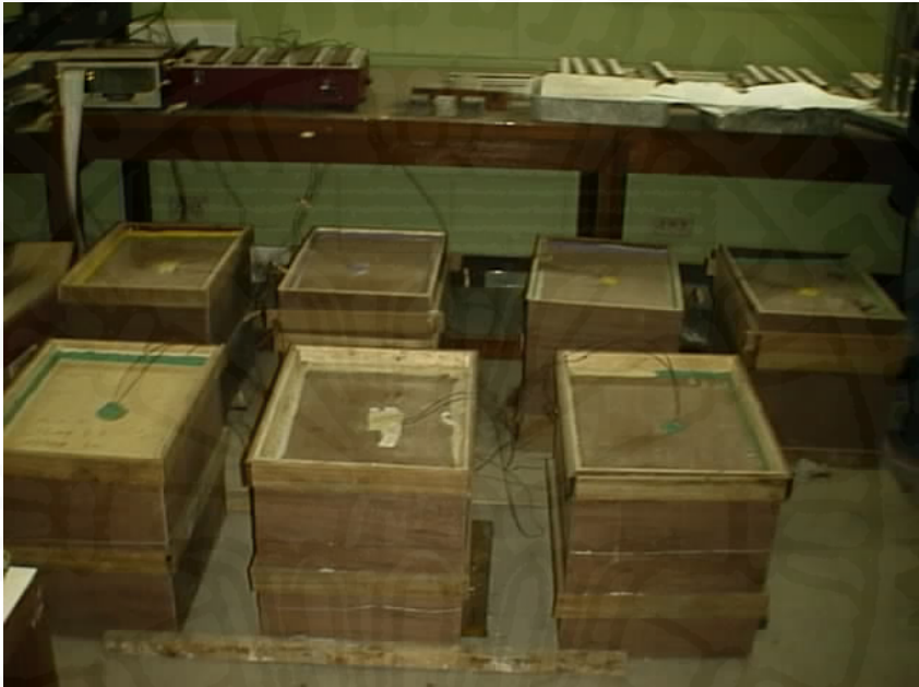
Fig 8.4 Testing of semi-adiabatic temperature of concrete
