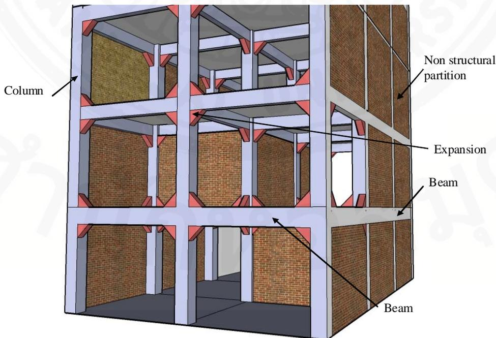
Fig. 1.3 3D Building beam-column frame system retrofitted with planar joint expansion
