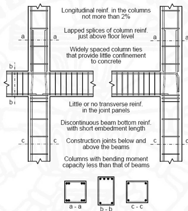
Fig. 1.2 Typical details in under-designed reinforced concrete structures.
