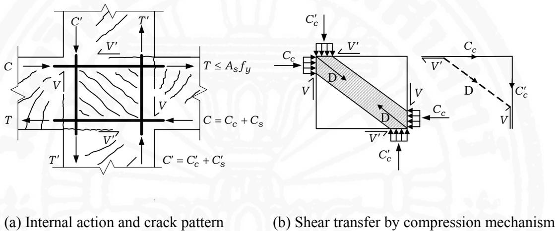
(a) Internal action and crack pattern
