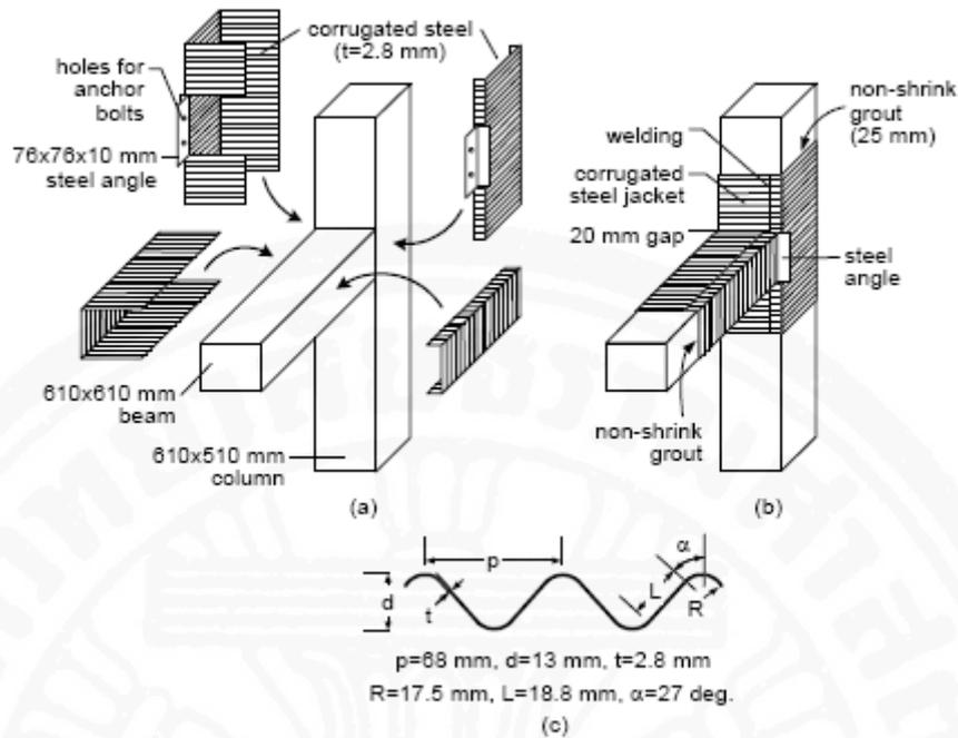
Fig. 2.11 Corrugated steel jacketing technique proposed by Ghojarah et al. (1997) and Biddah et al. (1997): (a) before installation, (b) after installation, (c) cross-section of the corrugated steel plates.
