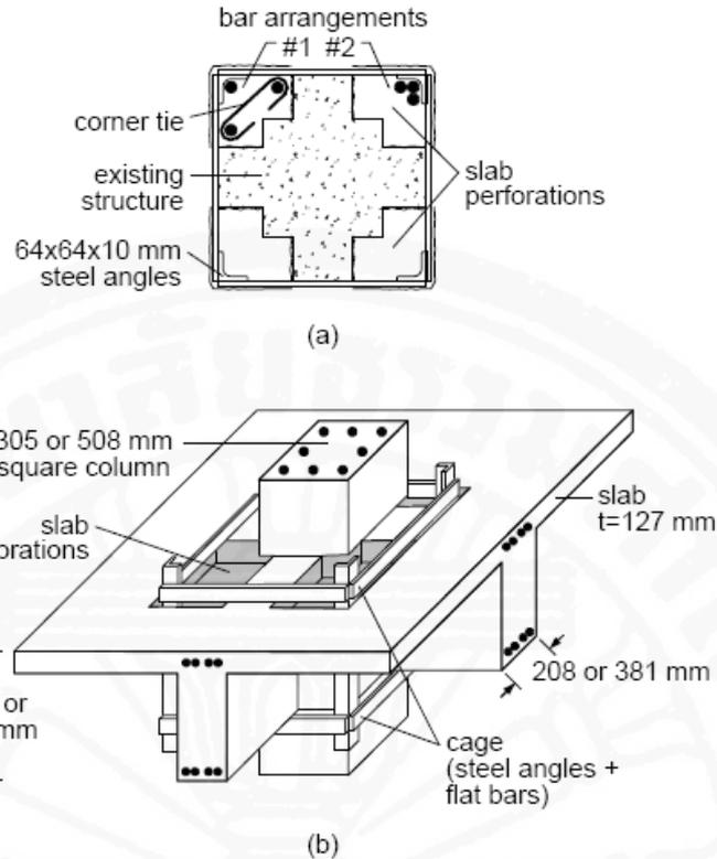
Fig. 2.4 Concrete jacketing technique studied by Alcocer and Jirsa (1993)
