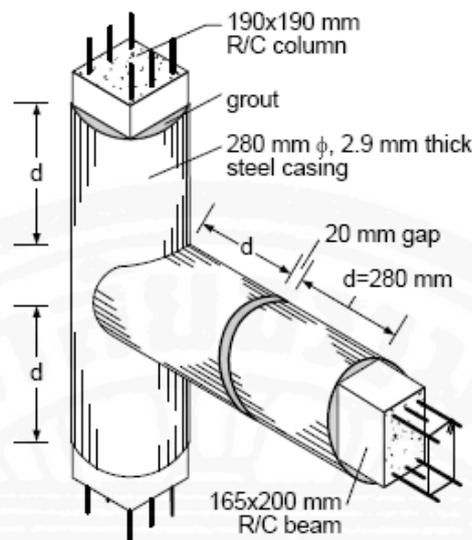
Fig. 2.10 Grouted steel tube technique studied by Hoffschild et al. (1995).
