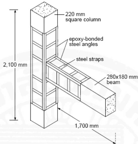
Fig. 2.6 Typical exterior joint strengthened with a steel skeleton by Migliacci et al (1983).
