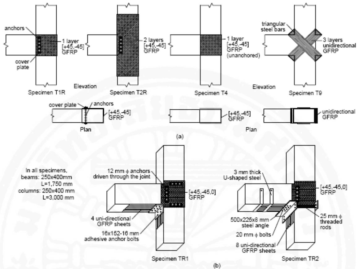
Fig. 2.14 GFRP-strengthened specimens tested by (a) Ghojarah and Said (2002), (b) El-Amoury and Ghojarah (2002)
