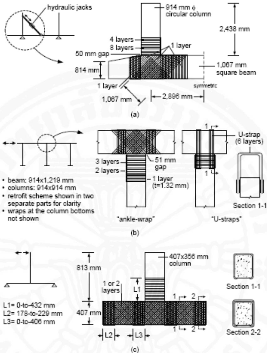
Fig. 2.12 CFRP-strengthened bridge bents tested by (a) Gergely et al. (1998), inverted bridge bent laboratory test, (b) Pantelides et al. (1999) and Pantelides and Gergely (2002), bridge bent tested in the field, (c) Gergely et al.(2000), inverted laboratory test.
