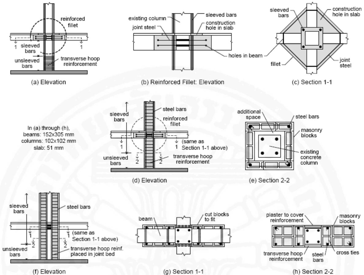
Fig. 2.5 Retrofit techniques studied by Bracci et al. (1995): (a, b, c) prestressed concrete jacketing, (d, e) masonry block jacketing, (f, g, h) partial masonry infill.
