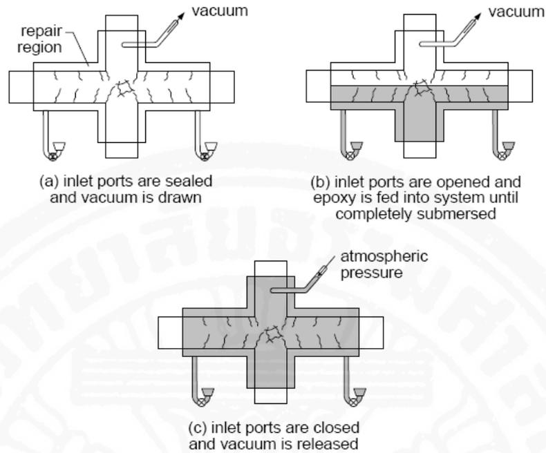
Fig. 2.3 Vacuum impregnation procedure applied by French et al (1990)
