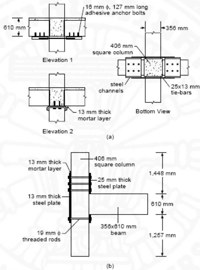
Fig. 2.8 External steel configurations studied by Beres et al (1992).
