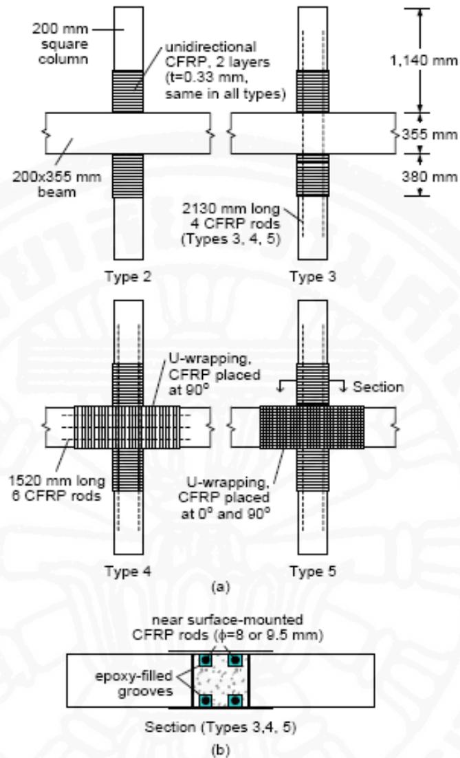
Fig. 2.13 Specimens strengthened with CFRP sheets and/or rods, tested by Prota et al. (2001; 2002): (a) elevation, (b) plan.
