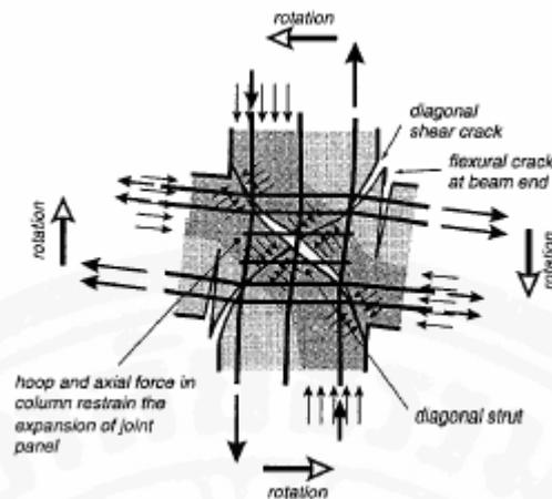
Fig. 2.2 Behavior model for joint shear failure and force flow in beam-column connection (Source: Shiohara, 2001)
