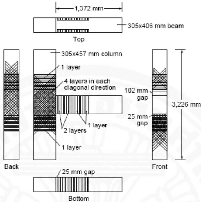
Fig. 2.15 CFRP-strengthened specimen tested by Cylde and Pantelides (2002)
