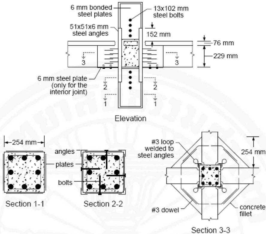
Fig. 2.7 External steel configurations studied by Corazao and Durrani (1989).
