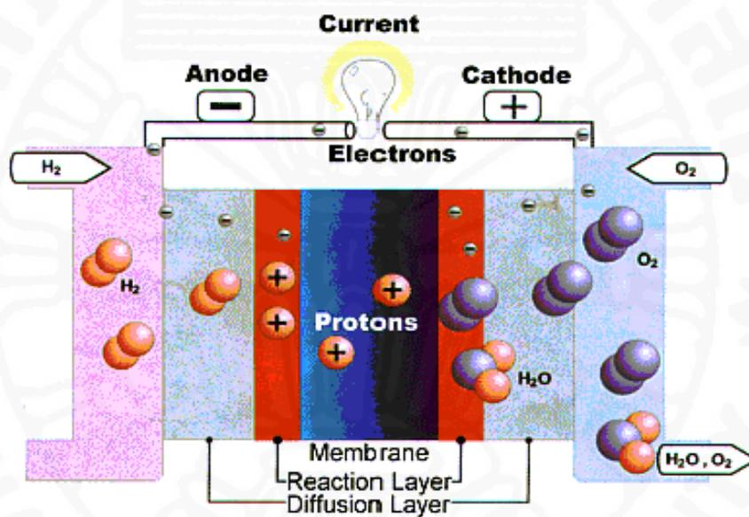
**Figure 1** Schematic of hydrogen fuel cell
