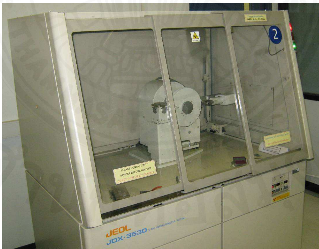
Figure 18 X-ray diffractometer (JEOL, JDX-3530)
