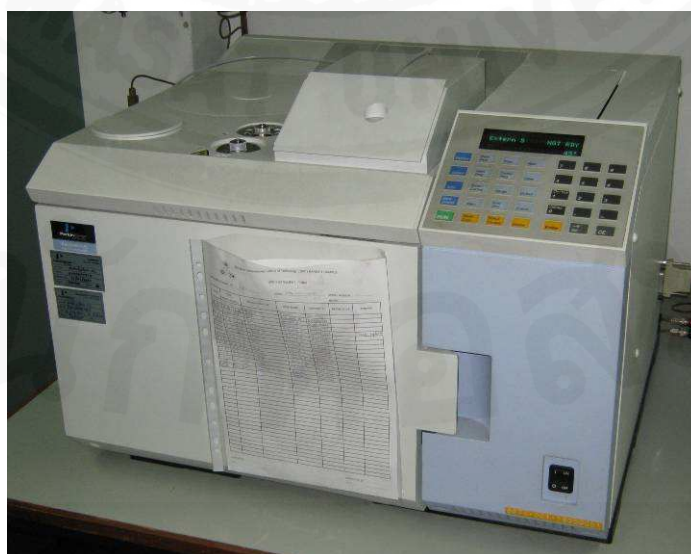
Figure 14 Gas chromatograph (Perkin Elmer- Autosystem XL)
