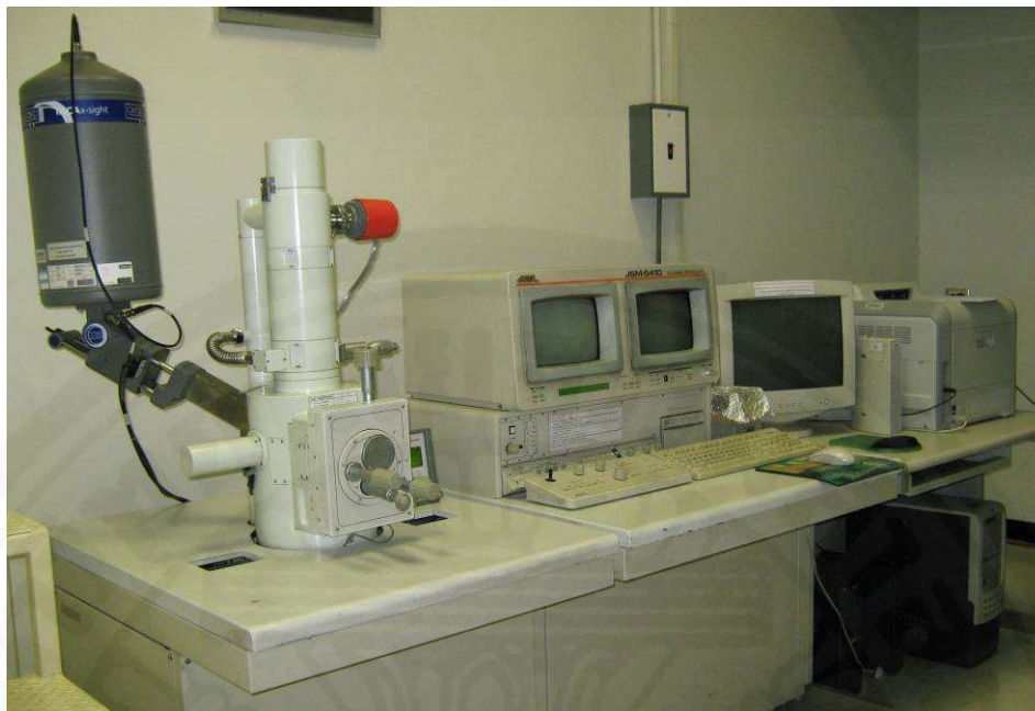
Figure 16 Scanning electron microscope (JEOL JSM-5410)
