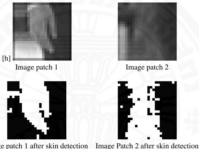
Figure 5.4: Both image patch 1 and 2 are classified as hand by the boosted classifier cascade. Skin detected images of those two images are shown below each of the images. Boundary feature extracted from skin detected binary image helps in elimination of this kind of false detection.
