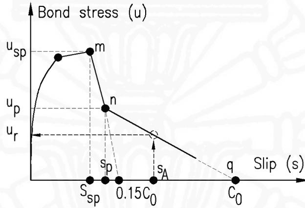
Fig 3.5: Calculation of bond stress for a specific slip  $s_A$
