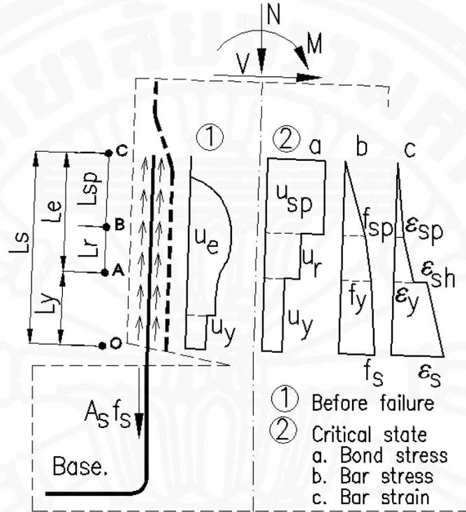
Fig 3.1: Tri-uniform bond stress model
