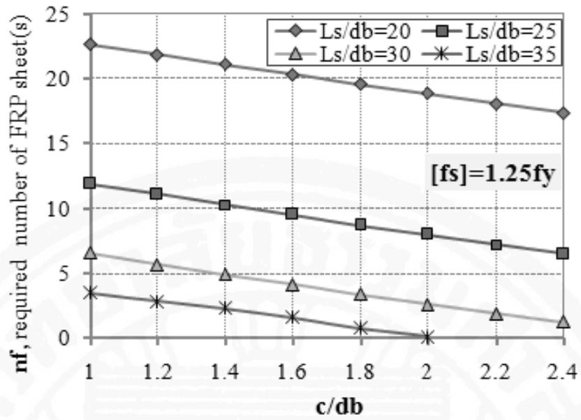
Fig 3.16: Required FRP sheets versus  $c/d_b$
