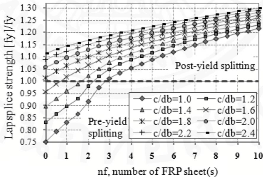
Fig 3.12: Strength of lap splice ( $L_s/d_b = 25$ )
