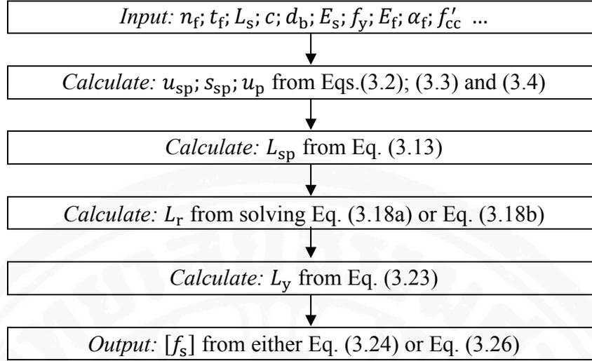
Fig 3.8: Calculation steps for lap splice strength
