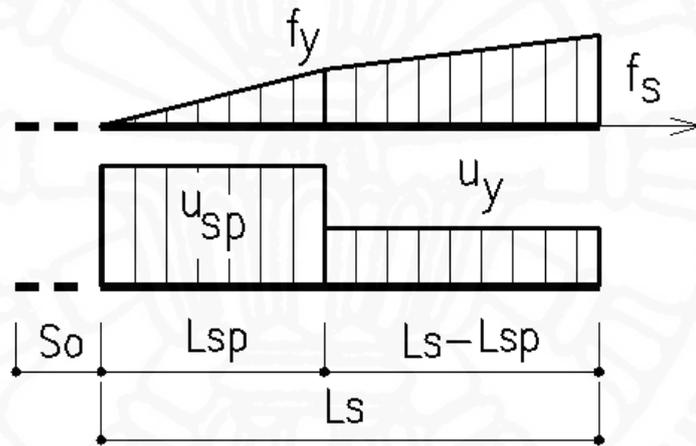
Fig 3.7: Free slip at the end of lap splice length
