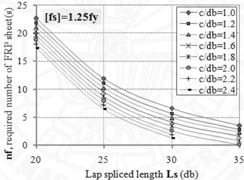
Fig 3.15: Required FRP sheets versus lap spliced length
