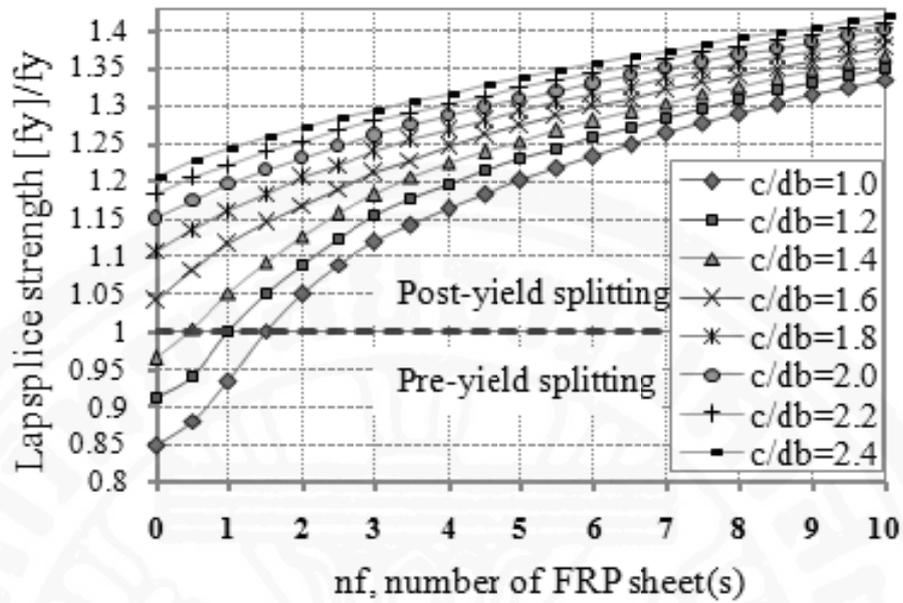
Fig 3.13: Strength of lap splice ( $L_s/d_b = 30$ )
