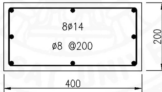
Fig 3.10: Column section used in parametrical investigation
