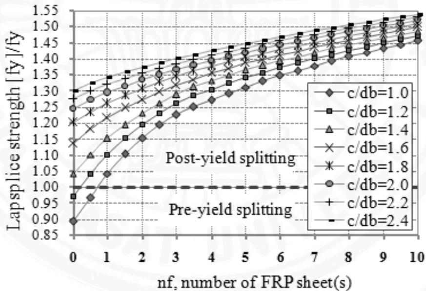
Fig 3.14: Strength of lap splice ( $L_s/d_b = 35$ )
