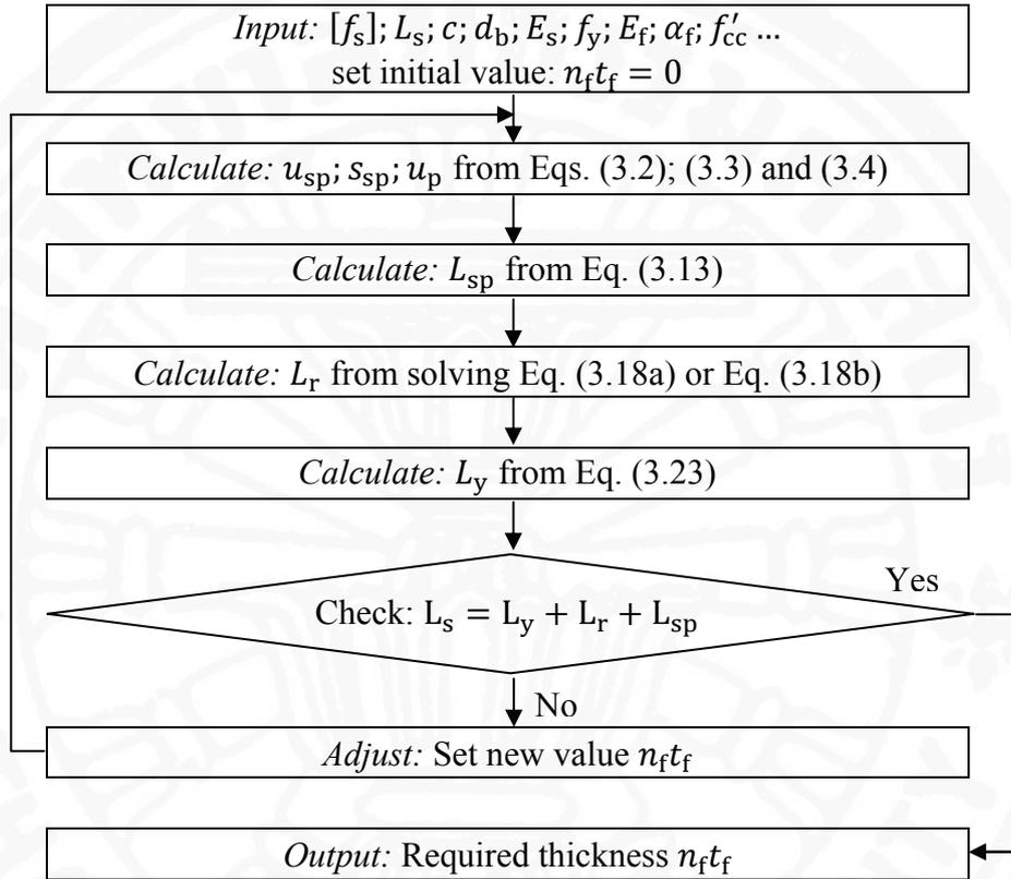
Fig 3.9: Calculation procedure for determining the required  $n_f t_f$
