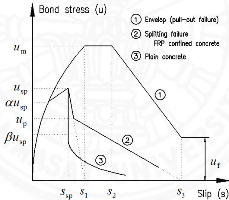
Fig 3.2: Bond stress-slip model by Harajli (2006)
