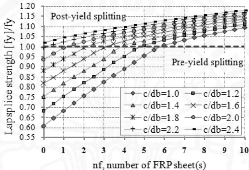
Fig 3.11: Strength of lap splice  $L_s/d_b = 20$
