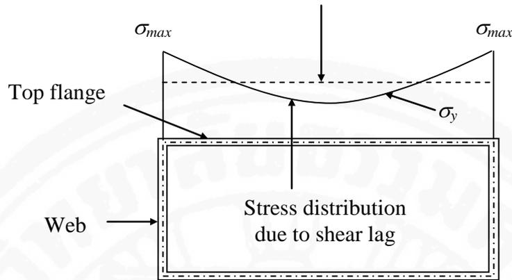
Figure 1.1 Stress distribution due to shear lag
