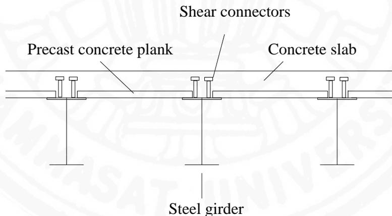
Figure 6.2 Composite steel-concrete bridge
