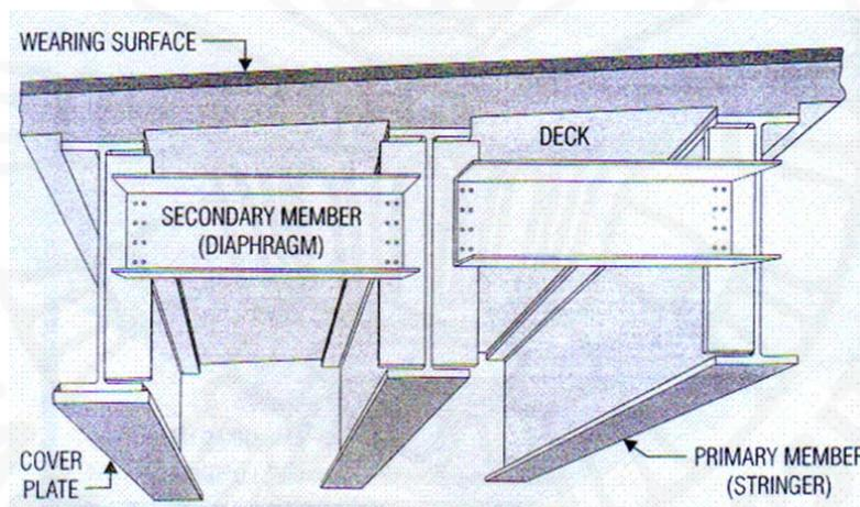
Figure 6.1 Principle components of a slab-on-stringer superstructure
