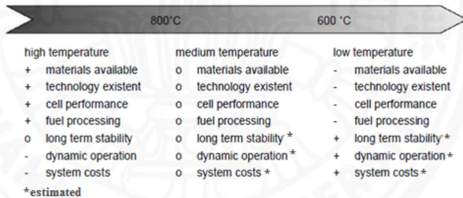
Figure 1.1 Advantages (+) and disadvantages (-) of SOFC for different operating temperature ranges, (o) designated states between (+) and (-) (Weber and Ivers-Tiffèe, 2004)
